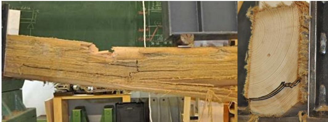
Figure 7: exemplary illustration of a combined failure – sample series „solid timber“; left: bending failure between the support and the load application; right: shear failure along the growth rings on the support of the same specimen
