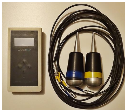
Figure 5: ultrasound measuring instrument Sylvatest Trio (CBT CBS, Lausanne/CH); left: measuring apparatus; right: measuring cables with transmitting and receiving probe
