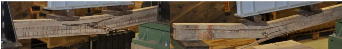
Figure 9: exemplary illustration of a combined failure – sample series „glulam“; left: bending failure in the centre of the specimen; right: combined failure with a bending failure beneath the load application and a shear failure along the glued joint
